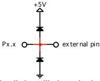
The diodes will short circuit any input voltages lower than 0V to ground and any higher than supply voltage to +5V.
