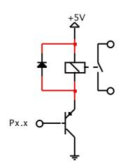
The same circuit may be employed if you want to control a DC electric motor. Any inductive load has the bad behaviour of generating a voltage with reverse polarity upon being switched off. If this is not shorted with the diode the voltage will rise to relatively high levels that can damage the driver transistor and/or the IO-Warrior.
