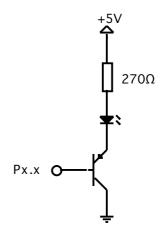
The LED may be the LED of an opto coupler. It may be necessary to adapt the value of the resistor to the LED or optocoupler you use.
